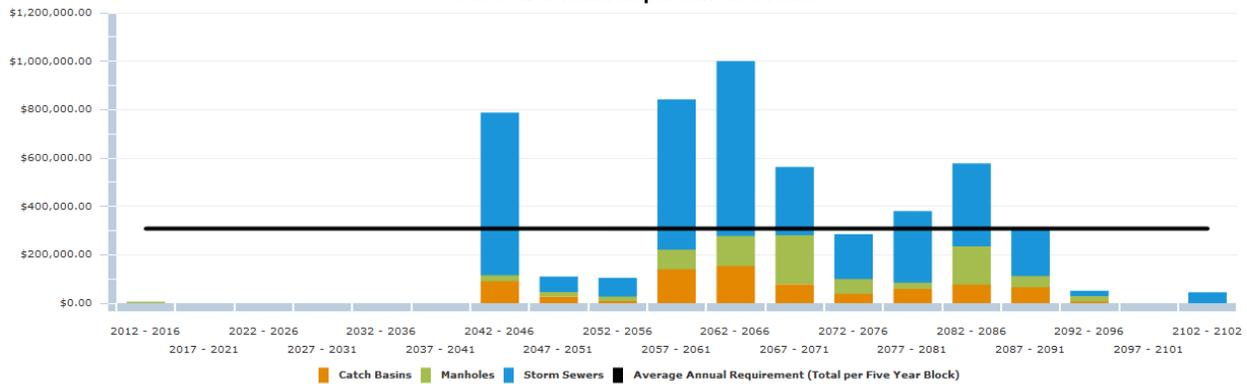
In conclusion, the storm sewer network, from an age based analysis only, is generally in Fair to Good condition and there is not a significant amount of replacement required for some decades into the future. It should be noted, however, that a condition assessment program would outline any pipes that have accelerated deterioration and could be good candidates for a rehabilitation program. This is discussed further in the Asset Management Strategy portion of the Asset Management Plan.
